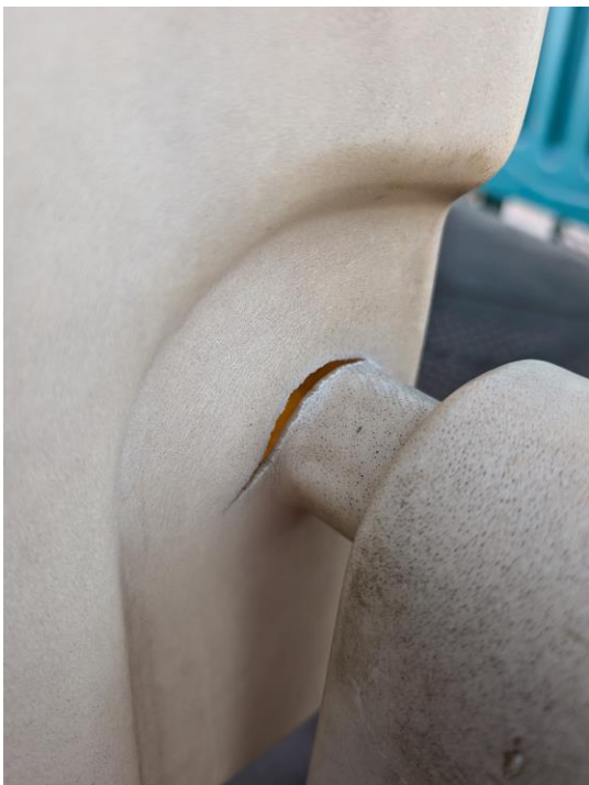
Top of slide detaching from the structure
