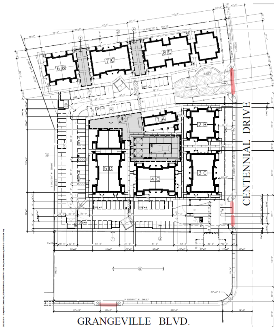
Figure 7: Site Access (shown in red)
