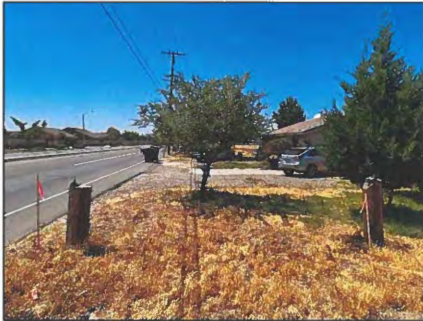
View looking south along the take areas from the property's northern boundary. The two surveyor stakes identify the new ROW taking.
