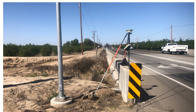
Existing USGS benchmark near proposed B.M. 196 location, Surveyed by Provost & Pritchard in March, 2021
