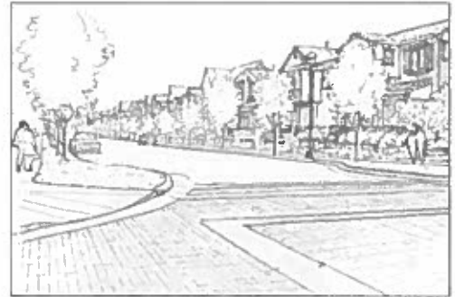
Paving materials at residential intersections let drivers know they are entering an intersection and adds richness to the streetscape
