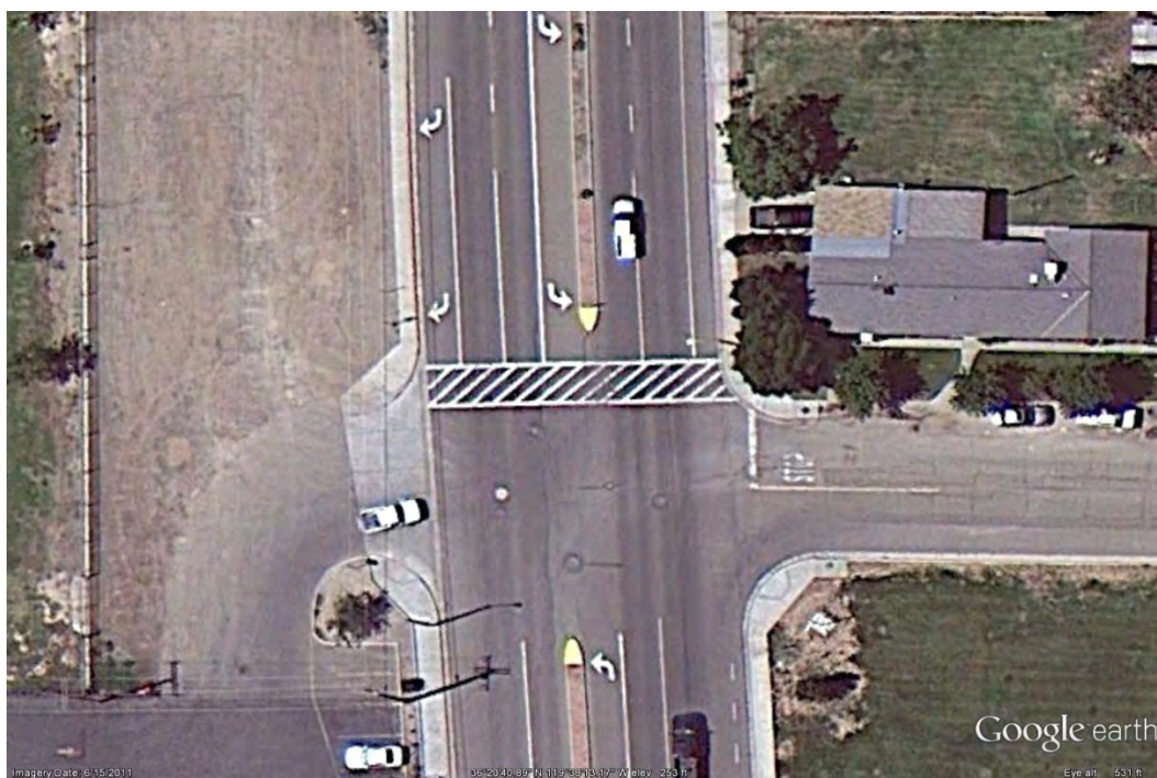
b) Slanted high visibility crosswalk
