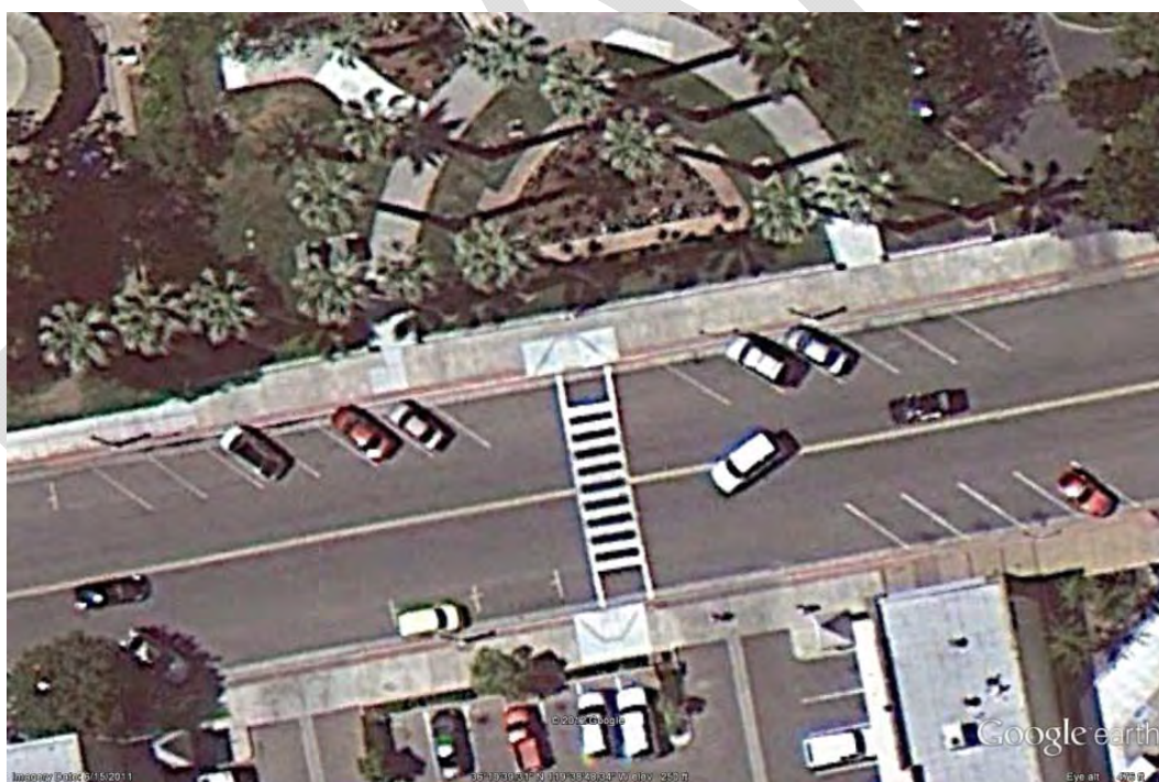
c) Vertical high visibility crosswalk
